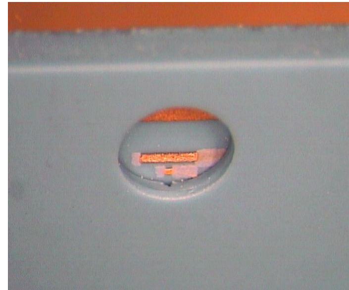
Fluidic interconnection at 100 \mu m channel
