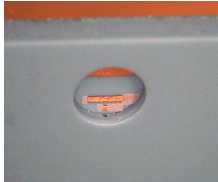
Fluidic interconnection at 100 \mu m channel
