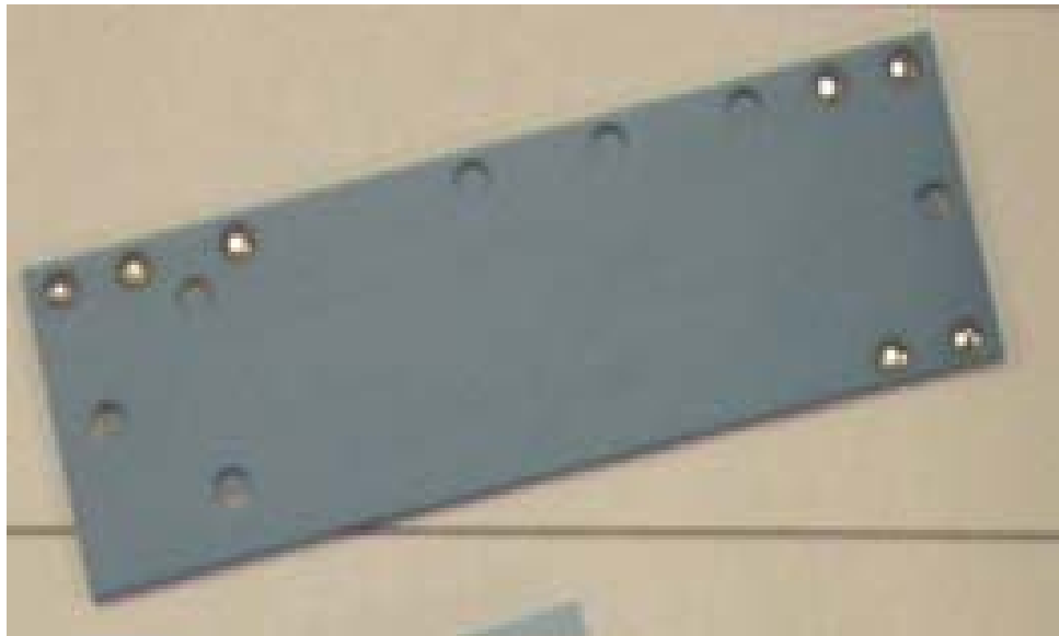
Fluidic Chip with integrated high voltage conductors
